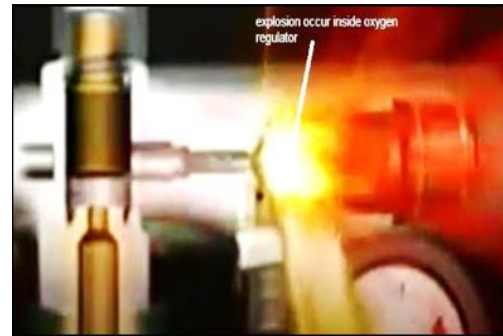
Figure 7: The accumulation of heat inside regulator lead to valve or cylinder explosion.
