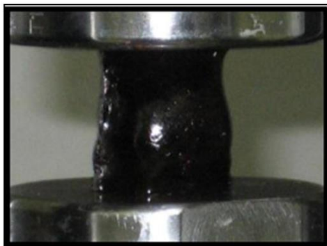
Figure 5: Experimental setups for compression testing (left) included preparing right circular cylinders 25 mm in diameter and 30 mm in height and compressing samples using an instron model 5567. Calculated stresses and strains were used to determine elastic modulus. Nanoindentation (right) used samples 1 cm in diameter and 1 cm in height. Samples were indented using a 90° conical PMMA tip, indenting 10 \mu\text{m} depth. Stiffness was calculated as the slope of the tip removal curve between 40-90% strain.
