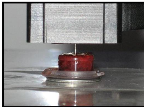
Figure 5: Experimental setups for compression testing (left) included preparing right circular cylinders 25 mm in diameter and 30 mm in height and compressing samples using an instron model 5567. Calculated stresses and strains were used to determine elastic modulus. Nanoindentation (right) used samples 1 cm in diameter and 1 cm in height. Samples were indented using a 90° conical PMMA tip, indenting 10 \mu\text{m} depth. Stiffness was calculated as the slope of the tip removal curve between 40-90% strain.
